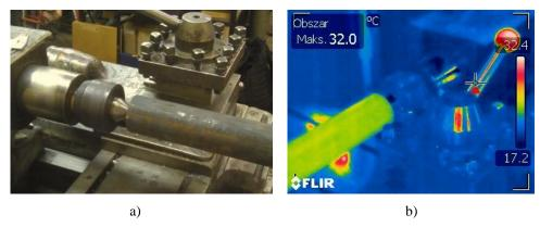
Fig. 2. Thermal imaging laboratory stand: a) the cast iron shaft mounted in the TUD50 lathe, b) thermography image taken with FLIR 335 camera in room conditions temperature
